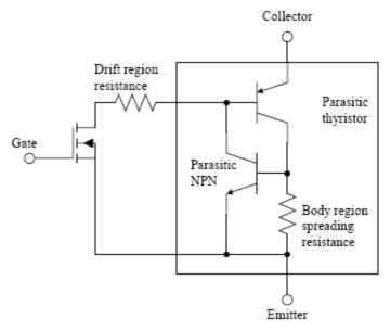
Figure 2: Equivalent Circuit of IGBT
